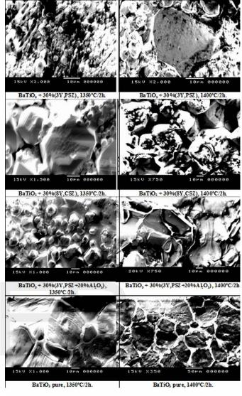
Figure 2. SEM micrographs of the sintered samples.
