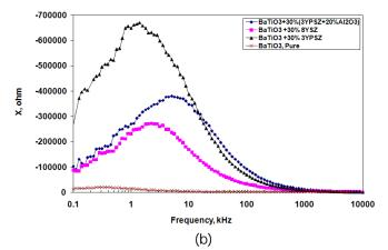
Figure 3. Impedance spectroscopy of the studied samples at 500oC.
