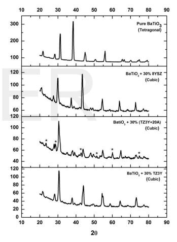
**Figure 1:** XRD patterns of the sintered barium titanate: pure and with 30 mol% of different additives sintered at 1350oC.
